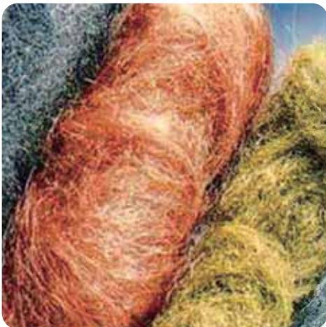
Ultra-thin Metal fibre, produced With COIL SHAVING METHOD
